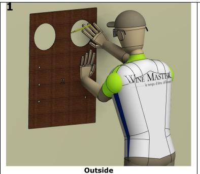
The template provided allows you to preview the size of the machine and draw the holes to be drilled. Please, note that if the appliance is placed on the floor, the template is intended for the minimum height of the feet.
