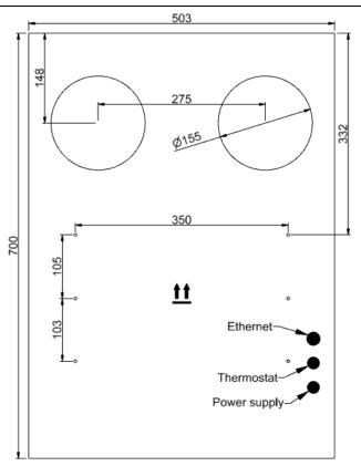
Place the drilling template against the exterior wall where the WINEMASTER  $\!\!\!\! \mathbb{R} \!\!\!\! \mathbb{R}$  air conditioner will be installed
